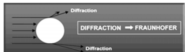
Figure 1: Behavior of laser beam obstructed by soil particle according to the Fraunhofer theory (Beatop Electric Limited, 2012)
